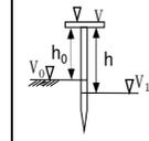
$h_1 = V_0 - V_1 = h - h_0$ (但し、 $h_0 = V - V_0$<br>$h = V - V_1$ ) |
